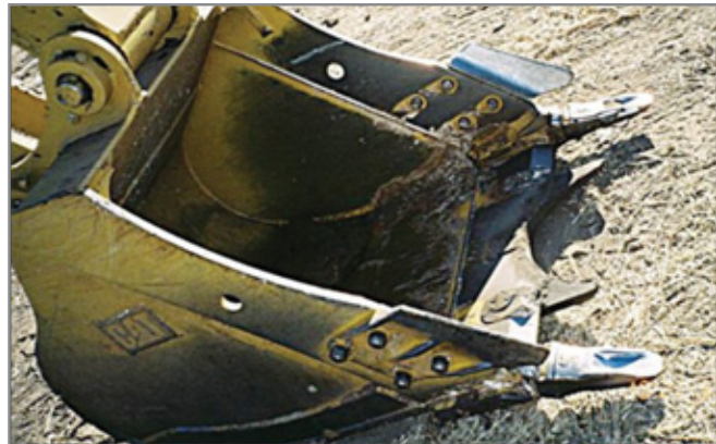
Half-moon spoon used to evacuate and conform 16" pipe.
